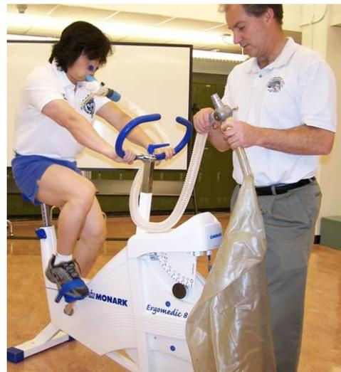
**Figure 4. The author using a Douglas bag to collect expired air from a student riding a Monark cycler ergometer.**
