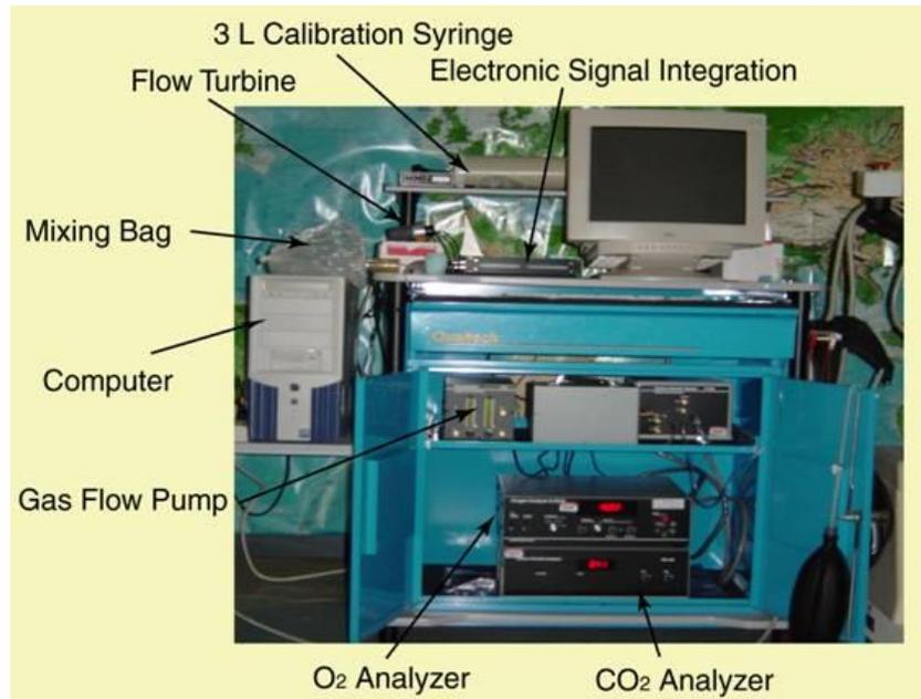
**Figure 1. Equipment used in expired gas analysis indirect calorimetry (EGAIC), consisting of a flow turbine, expired gas mixing chamber/bag, gas flow pump, electronic gas analyzers for oxygen and carbon dioxide, a means to remove moisture in the expired gas, and of course computer hardware and software to run the system.**
