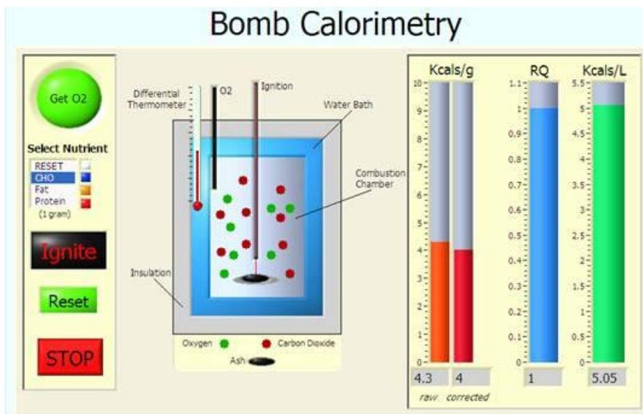
Figure 1. Illustration of the bomb calorimeter, with added features to highlight measurements and results for energy of combustion for carbohydrate.
