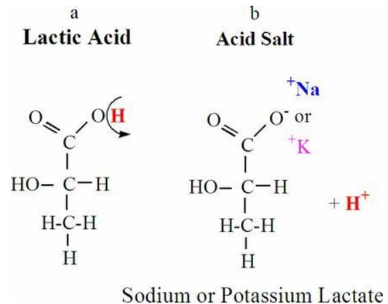
**Figure 1. The chemical structures of a) lactic acid vs. b) lactate.**
