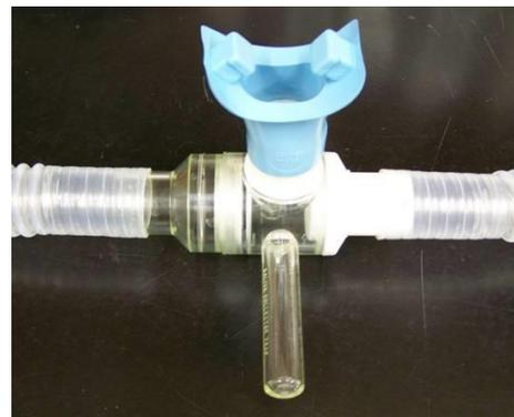
**Figure 7. Photograph of the one-way T-valve apparatus connected to inspired and expired low resistance tubing.**
