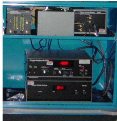
**Figure 17. Electronic expired gas analyzers used in our custom-developed system.**
