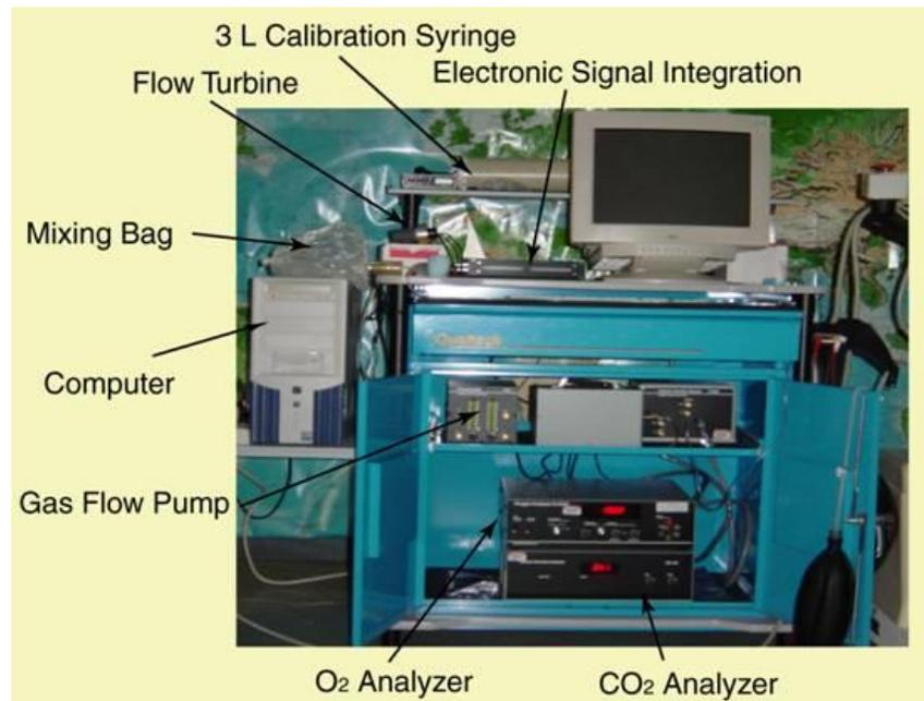
Figure 4. Photograph of a custom indirect calorimetry system developed at the University of New Mexico.
