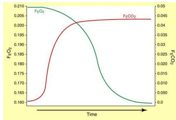
Figure 20. The time dependence for the change in expired oxygen ( $F_{EO_2}$ ) and carbon dioxide ( $F_{ECO_2}$ ).
