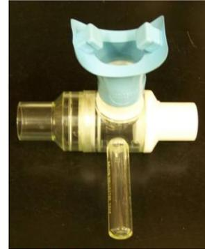
**Figure 5. Photograph of a one-way T-valve apparatus.**
