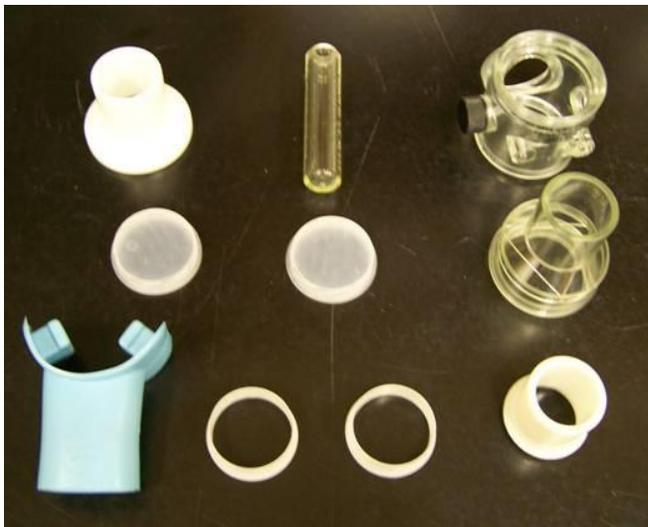
**Figure 8. Photograph of the individual components of a one-way T-valve apparatus.**
