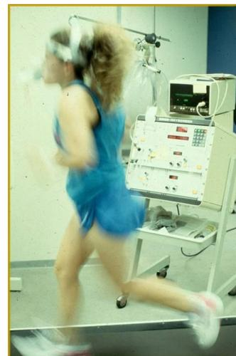
Figure 15. The expired air pneumotach, which in this example, is located just prior to the mixing bag to the left of the ECG unit.
