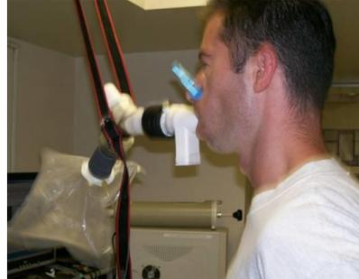
Figure 11. A subject exercising using a custom developed compliant mixing chamber fitted to the expired side of a "Y" shaped one-way valve apparatus.
