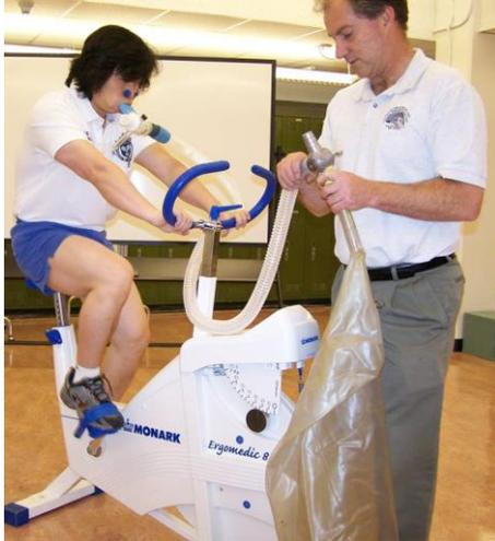
Figure 13. Use of the Douglas bag to collect expired air.
